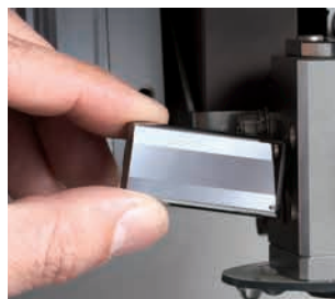
Power Feed Contact
